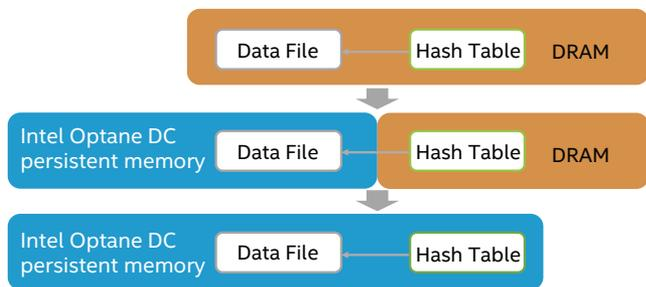
**Figure 4** Baidu Feed-Cube Memory Hardware Change Path
